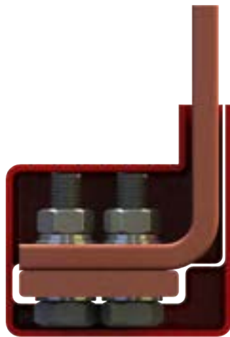
Cut-Section of the product mounted on the busbar assembly
