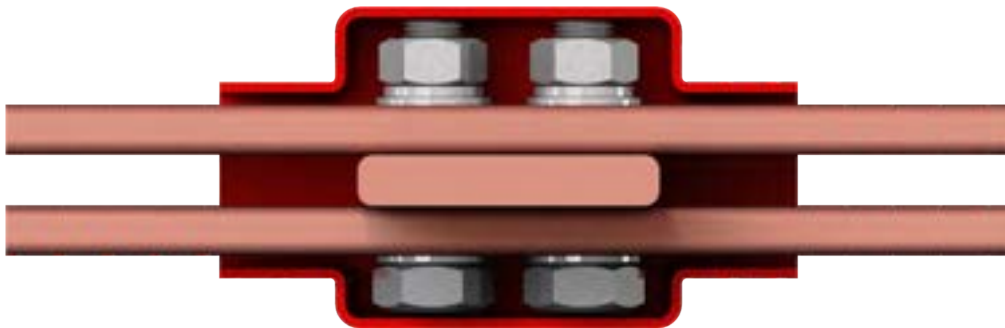
Cut-Section of the product mounted on the busbar assembly
